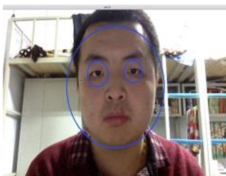
图4 强光下定位人脸及人眼结果 Fig.4. positioning human face and eye results with strong light
