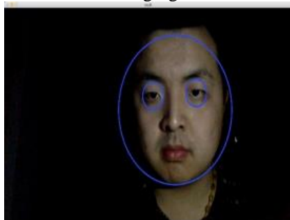
图5 弱光下定位人脸及人眼结果 Fig.5. positioning human face and eye results with weak light
